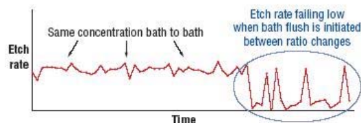
Figure 1. Improper draining of bath causes low etch from diluted acid.
